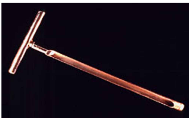
Figure 4. "T" type sampling tools are ideal for collecting most types soil samples for nematode analysis.
